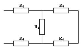
$R_1 = R_3 = 100 \Omega$ ;  $R_2 = 150 \Omega$  et  $R_4 = 500 \Omega$ .
